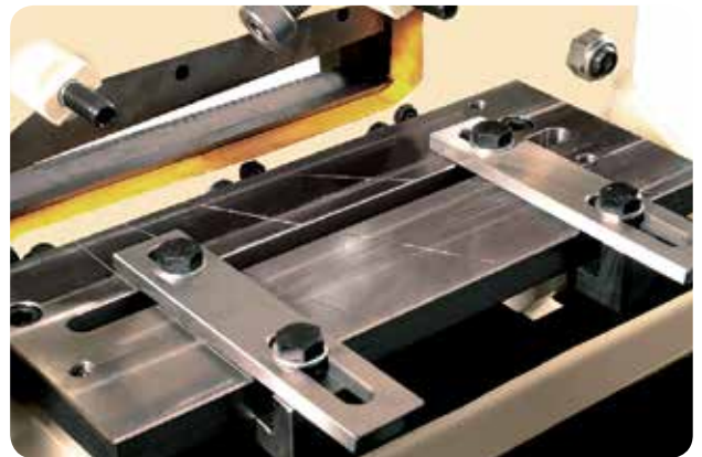
3 In order to eliminate permanent deformation in material during the cutting process, the BENDICROP range includes an exclusive DEFORMATION-FREE CUTTING SYSTEM. This system is specially designed to cut soft materials (copper, aluminium), with spectacular cutting finishes.
