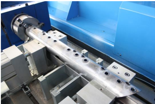
Round tube with 4 axis, set-up <5 minutes
