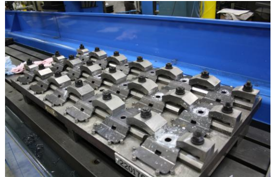
Multiple clamping of small parts on jig
