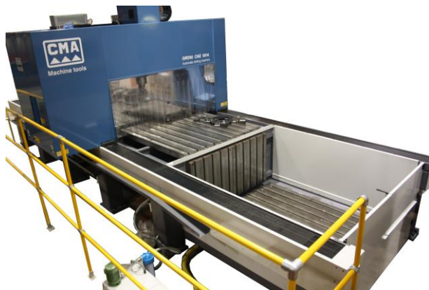
GRD 6514 (X/Y 6,5 x 1,4 m) 2 table-heights and vertical table, spindle-table 660 and 1480 mm
