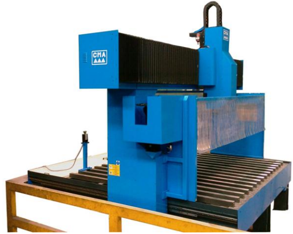
GRD (X/Y 3 x 3 m, spindle-table 1100 mm)
