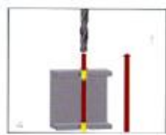
drilling profiles with intermediate rapid-feed
