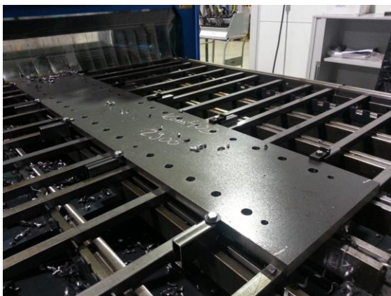
30 mm material, 46x \phi 26 mm + 12x \phi 14 mm 10 minutes 51 seconds with AMEC GEN3 tooling
