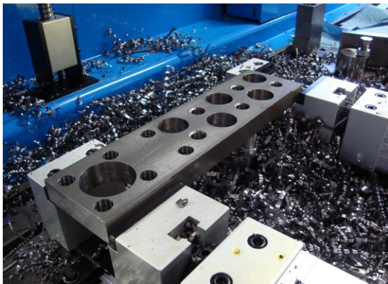
Drilling 21, 35 and 60 mm, tapping M24
