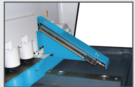
SAFETY LIGHT CURTAIN GUARDS in front of the hold-downs. BALL TRANSFERS mounted in the iron table blocks, for easy feed-in of the sheets.
